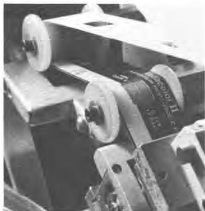
*Labels for cartridges to be loaded with Kodacolor II film are fed to the film spooling machines.*
