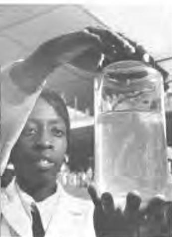
*Clear, honey-like liquid called "dope" is carefully checked by a technician for contamination.*
