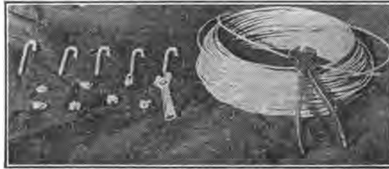
A roll of seven-strand galvanized cable (three-sixteenths of an inch in diameter), lag screw hooks and clips for fastening cable ends. The lag screws are inserted as far as possible so that the cable will not slip out of the hook.
