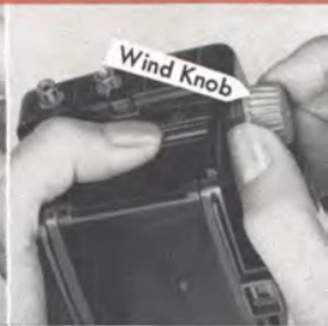
**3** Break film seal. Place end of spool in hook of spring under shutter release. Push down spool, swing it in until the end snaps into the hole.
