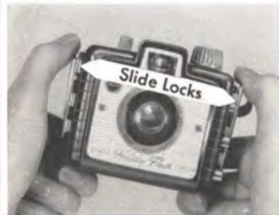
**1** Push the SLIDE LOCKS on both sides of the camera all the way down. Remove the camera back.
