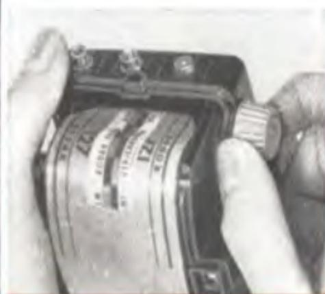
**4** Draw paper, colored side up, over opening; thread it through slit in spool as far as it will go. Wind two full turns to make sure paper is tight and straight.
