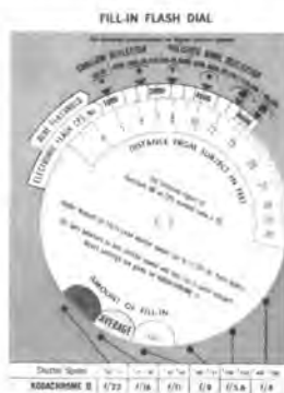
The Fill-in Flash Computer in the KODAK Master Photoguide simplifies exposures for fill-in flash.
