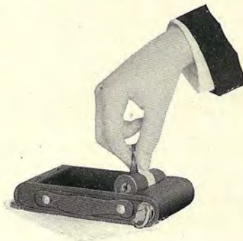
Fig. 2 Lifting out roll of exposed film.
