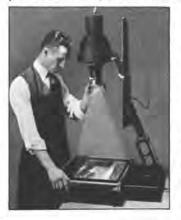
cupped supports for film in strips, takes negatives up to 21/4 x 21/2 inches (or 21/4 x 31/4 inches, masking off a 21/4 x 21/2-inch area). Special focusing target on negative carrier has sharp, fine-line pattern which can be slid into field of view temporarily in enlarging from negatives difficult to focus on account of their density. Enlarger regularly gives prints up
