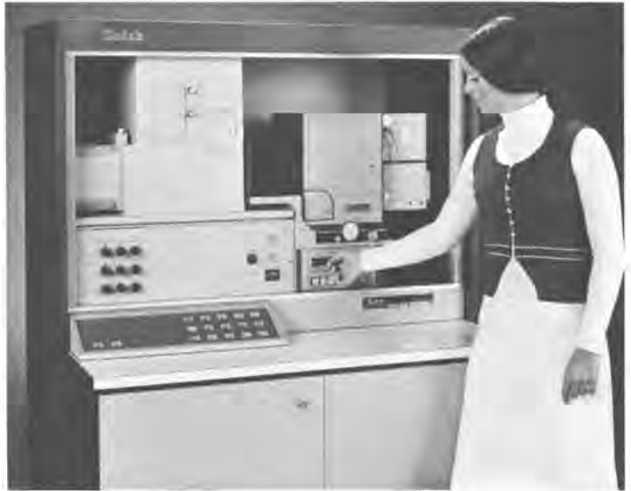
At speeds up to 120,000 characters per second, the KODAK KOM-80 Microfilmer transfers computer data directly onto microfilm.
