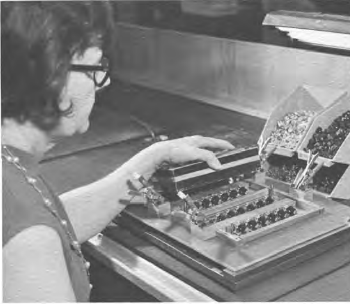
This special loading station prepares electronic exposure-control parts for wave soldering, a technique that solders many components in one rapid operation.
