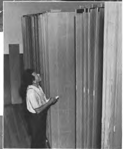
Photography as an implement of aircraft-manufacture: the Eastman Matte Transfer process. At the top, a machine laminating the photosensitive material to metal sheets. At the right, inspecting master templates made by the photographic process that has expedited the pattern stage in producing planes. Below, the finished product: in this case a North American B-25 bomber, the type that raided Tokyo
