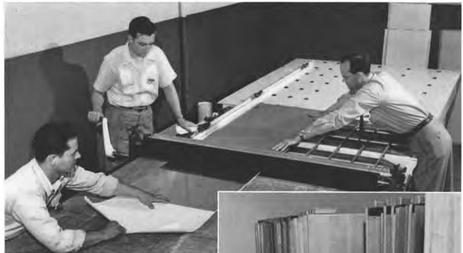
Photography as an implement of aircraft-manufacture: the Eastman Matte Transfer process. At the top, a machine laminating the photosensitive material to metal sheets. At the right, inspecting master templates made by the photographic process that has expedited the pattern stage in producing planes. Below, the finished product: in this case a North American B-25 bomber, the type that raided Tokyo
