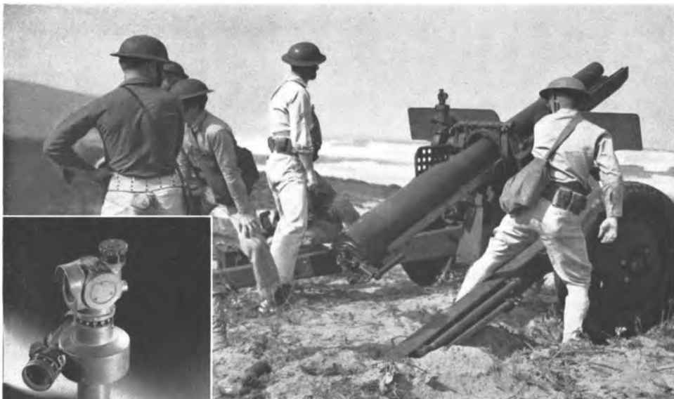
An M-12 panoramic telescope , used to sight this modern beach-defense gun in Hawaii, is seen mounted on the gun, and also in close-up. The Company manufactures the M-12 in large numbers
