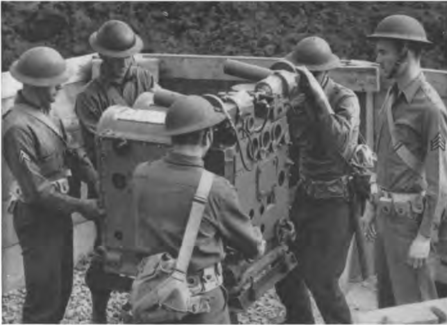
This intricate computing mechanism receives data from the height-finder and other sources . . . and directs the aim of anti-aircraft guns. It contains 25 high-precision subassemblies made by the Company. Eastman optical departments also provide "optics" for telescopes like those shown on the director Press Association
