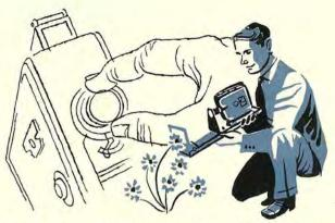
I F YOURS is a focusing camera with a lens that will barrel down so that you can approach to within 1 or 2 feet from objects, real close-ups are a cinch. For at 1 foot you can cover a field a bit less than 4 inches in width, and about twice that at 2 feet.
