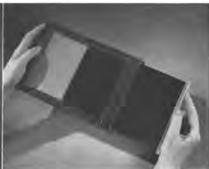
Step 5. Inserting dark slides with bright side out. Left thumb holds flap closed.
