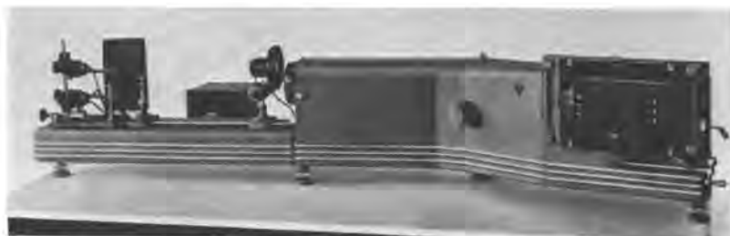
Medium Quartz Spectrograph, useful for general qualitative and many of the simpler types of quantitative analysis. Courtesy Bausch and Lomb Optical Company.
