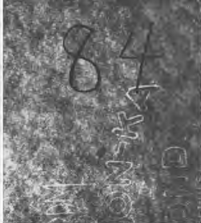
To show the texture and watermark of the paper, the specimen was illuminated from behind and photographed, with the above results.
