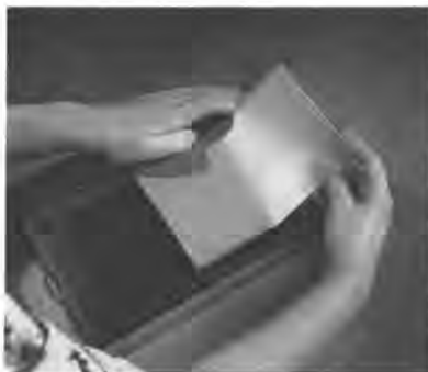
Step 4. Sliding film into channels of holder. Index finger on code notches.
