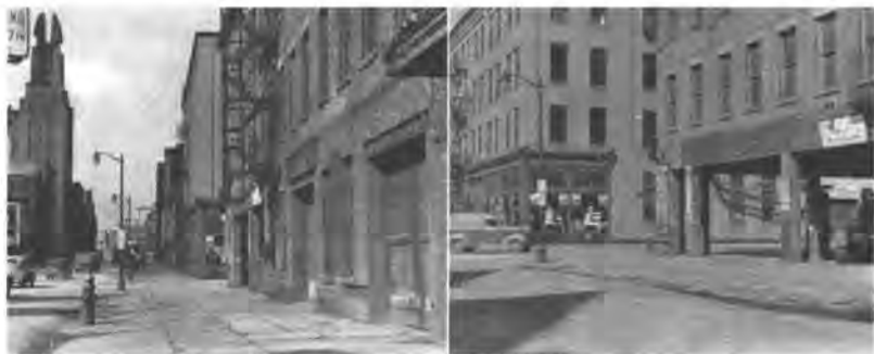
What appears to be a blind intersection in the photograph at left, is revealed to be a fairly open corner in photograph at right, taken from the driver's viewpoint.
