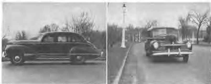
Automobile in photograph at left appears to be parked at the curb, but shifting the position of the camera reveals wide separation between automobile and curb.
