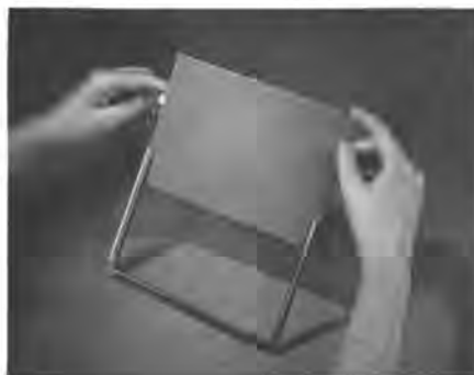
Loading film into developing hanger.
