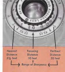
When taking pictures of objects that are less than 5 feet away, measure the distance from the front of the lens to the subject.
