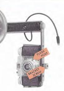
For flash pictures, use a Kodak flasholder. Remove the cap from the FLASH POST by pushing in and twisting it to the left. Connect the cord to the flash post and screw the BRACKET SCREW into camera tripod socket.
