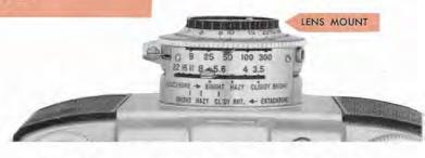
You'll get sharper pictures if you carefully estimate the distance in feet from the lens to the main subject; then set the lens at this distance. To bring the camera into focus, turn the LENS MOUNT until the camera-to-subject distance is opposite the focus-index mark.
