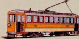
300 Series-Rebuilt Single Truck Cars, Three Windows Longer with Double Trucks
